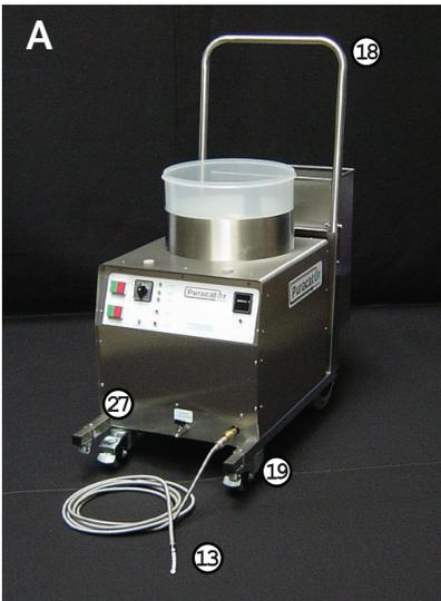
Puracator is fitted with fixed wheels at the rear and rotating and lockable front wheels (19) for easy but controlled manoeuvrability. The handles (18) are shown in the erect position (Photo A).
